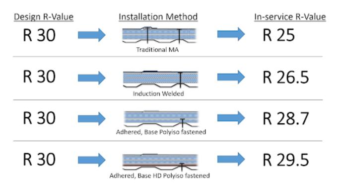
Figure showing In-Service R-value based on modeling a 15,000 square foot roof with a 120mph wind speed used to determine the fasteners quantities and densities.
