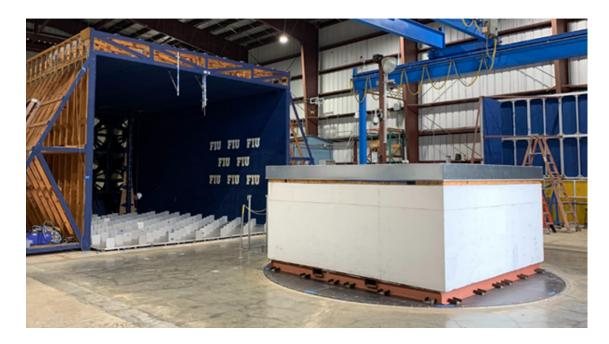
Importantly, FIU's WoW includes a turntable to which the test decks are mounted. The wind tunnel is capable of producing wind speeds up to 157mph in the free air stream, and the
