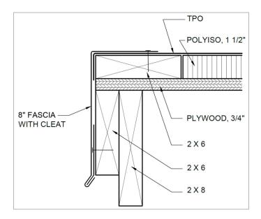
Two different 22-gauge steel cleat shapes were used—a 6 in. cleat and an 8 in. cleat with a 1 in. horizontal return (L-shaped cleats). Four different cleat-fastener locations were used—one low, one in the middle, and one high on the vertical surface, and one on the horizontal surface (Configurations #1, #2, #3, and #4, respectively). The figure below shows the 2 cleat shapes and 4 fastening locations used in this research.
