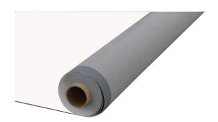
Parasolo TPX<sup>TM</sup> is a TPO single-ply membrane that incorporates a proprietary formulation of stabilizers and UV absorbers, offering enhanced heat-aging and UV weathering performance when compared to conventional TPO membranes.
